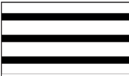
French drain, simple system: perforated pipes run in straight lines, the length of the arena.
